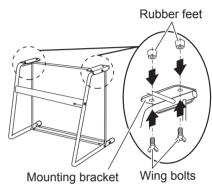
4) Provisionally place the unit on the stand's mounting brackets. After placing the unit on the stand, then working one bolt at a time, align each of the four holes on the bottom of the unit (the holes near the rubber feet) with the tip of the corresponding wing bolt, and tighten the aligned bolt securely.
