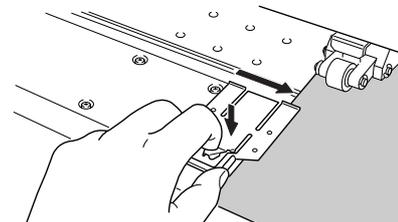
**3** Line up the holes in the media clamps with the left and right edges of the media.
