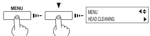
**3** Press the [▶] key, and press the [▼] key to display the screen shown in the figure.
