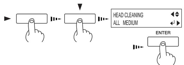
**4** When head cleaning finishes, perform a printing test to check the results.
