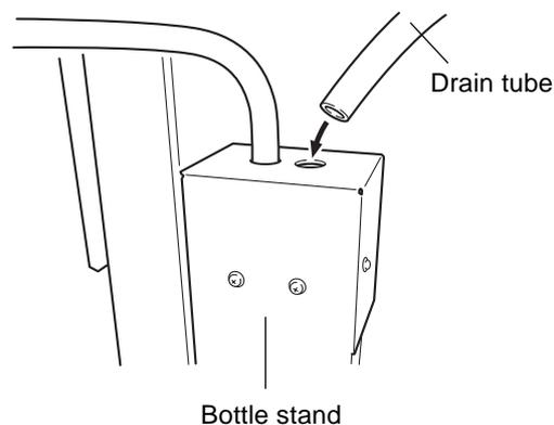
**4** Attach the drain bottle to the back of the machine.
