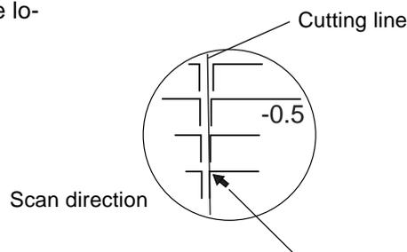
Read the scale on which the cutting line goes over as the correction-value .
