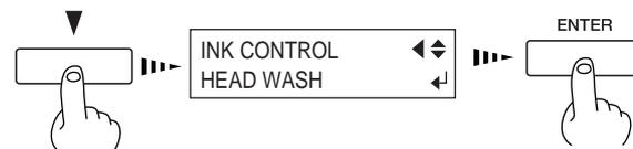
**5** When the display shown in the figure appears, discard the discharged ink in the drain bottle.
