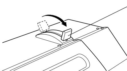
To secure the media in place, move all the way to "LOAD". When moved partway, only the left-hand pinch roller descends. Data cannot be output while in this state.
