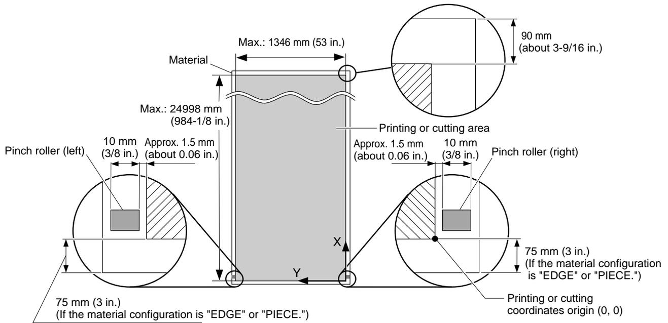
\* The arrows in the figure indicating the X and Y directions indicate respectively the positive directions of the X axis and Y axis.
