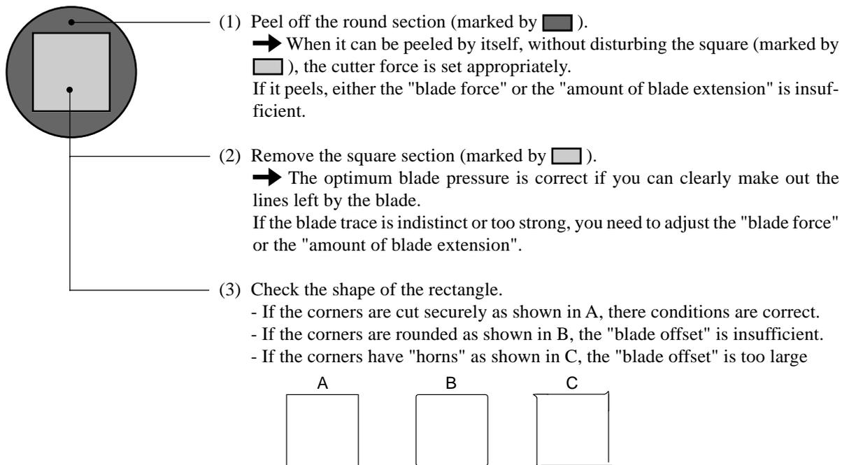
If the test cutting shows problems with the media cutting results, adjust the cutting conditions.
