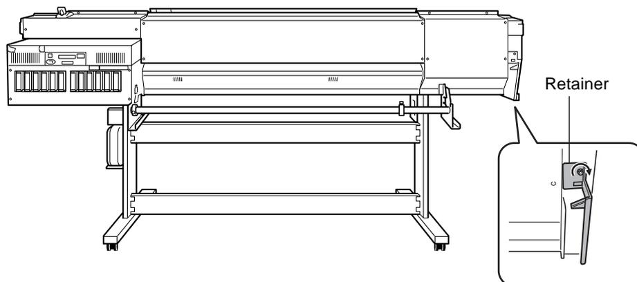
7) Attach the retainer you removed in step 4).
